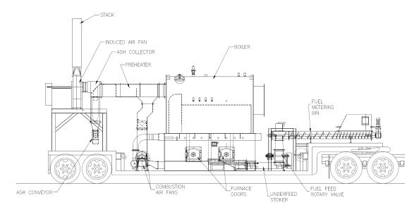
Solid fuel boilers can also be set up to be portable. This versatility proves to be convenient for users with seasonal hot water and/or steam heating applications.
