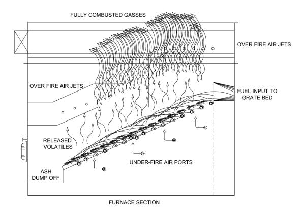
This schematic shows the process in which fuel enters the furnace and goes through the different stages of combustion.
