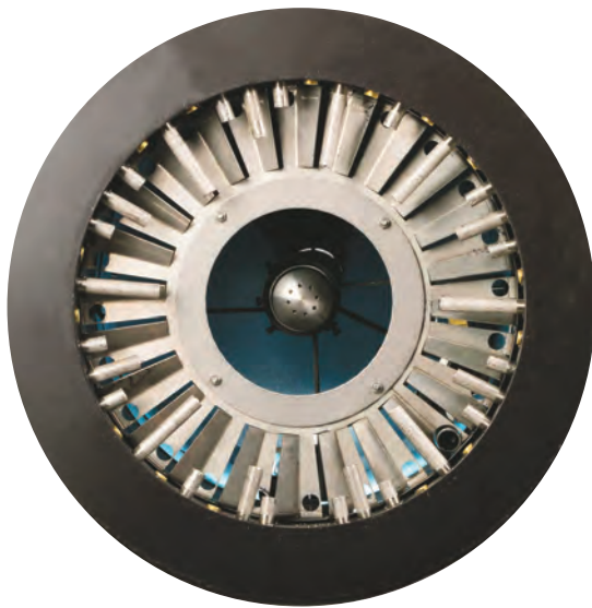
The high swirl burner head on the HDS(X) mixes fuel and air more efficiently.
