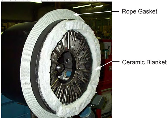
Figure B-14 Gas Manifold
