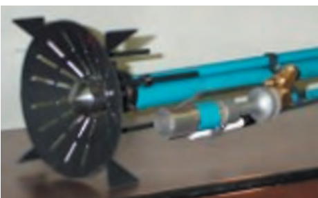
Figure B-11 Pilot and Diffuser
