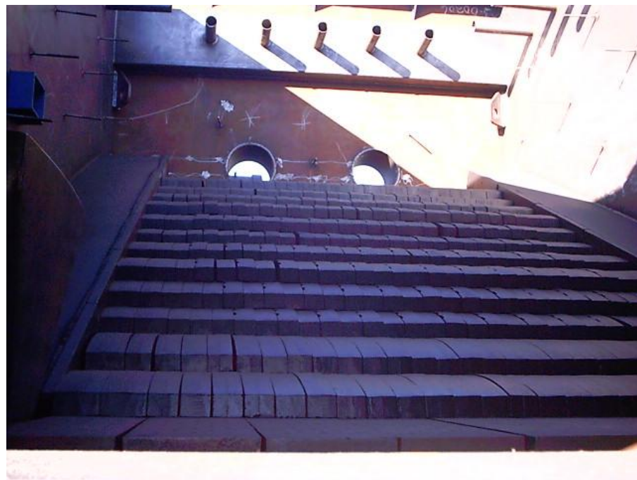
Figure 6 HBC's Automatic Deashing Biomass Stoker System
