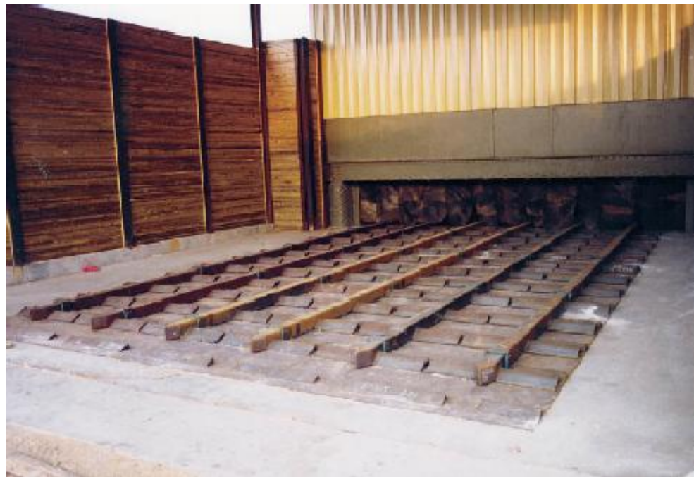
Figure 1 A typical reciprocating floor unit. Notice the main assembly is mounted on a single steel plate rather than to the concrete
